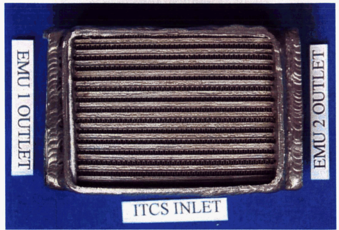
Figure 17. The ITCS passages of the dissected SPCU HX were visibly clean
