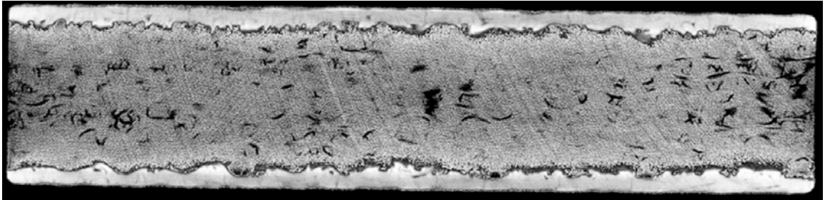
Figure 12. 100-micron scan taken at end of specimen where loading was very low.
