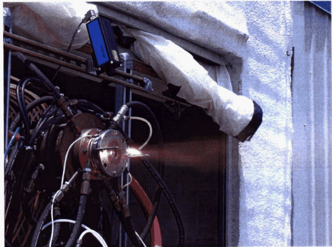
Figure 15. Temporary test configuration for pyrometry system check-out and environment reconnaissance.
