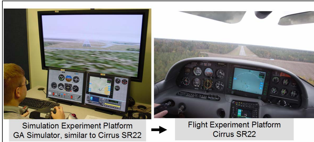
Fig. 4. HVO Experiment Platform Progression (note commonality of HSI and MFD)
