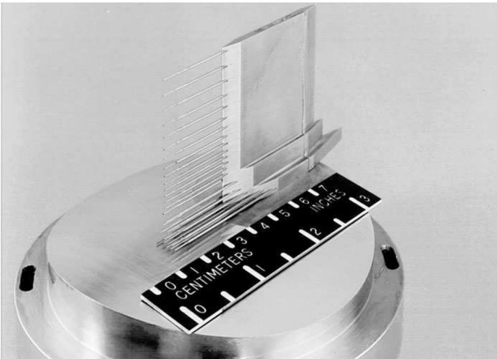
Figure 12. Concluded. (c) Boundary layer rake mounted on model plug.
