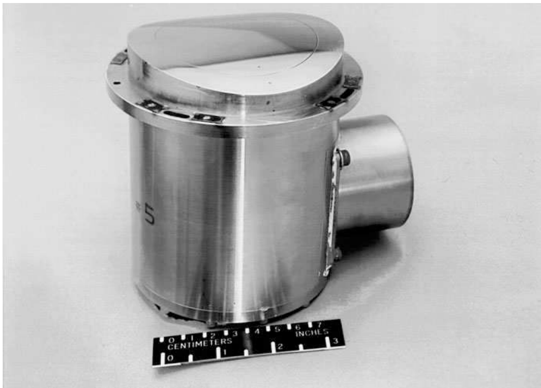
Figure 12. Instrumentation photographs. (a) Skin friction balance.
