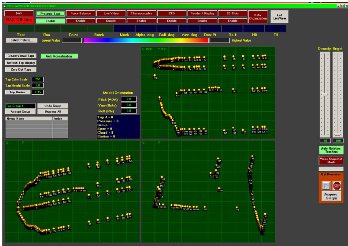
Figure 12. LiveView3D pressure tap user interface. Each pressure tap on the model is depicted as a yellow circle in the three two-dimensional projections of the virtual environment. Spatial coordinates for each tap are read directly from the virtual environment and mapped to scale. The user may select any number of taps to be in a group, and any number of groups can be created. To display the data in the virtual environment, the user has to enable a group.
