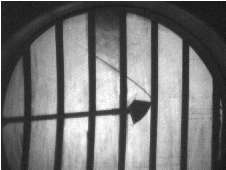
Figure 7. Schlieren image of the supersonic flow field about a model of the NASA Crew Exploration Vehicle in the LaRC UPWT. Vertical bars are slats that hold the test section windows in place.
