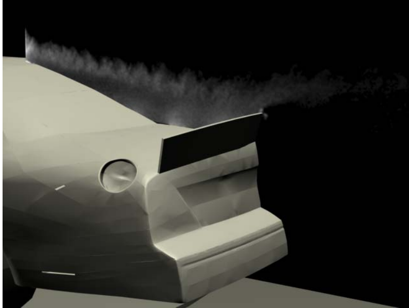
Figure 6. LiveView3D rendering of laser light sheet flow visualization over the rear deck of the stock car configuration.
