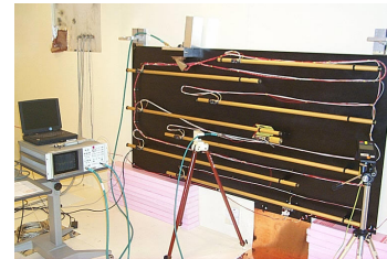
Figure 12. Laboratory set-up for arc/spark tests.
