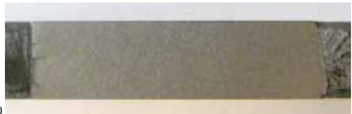
Figure 3— Photographs of representative fracture surfaces for C(T) specimens in lab air: (a) 76.2 mm wide, 12.7 mm thick; (b) 76.2 mm wide, 5.08 mm thick.
