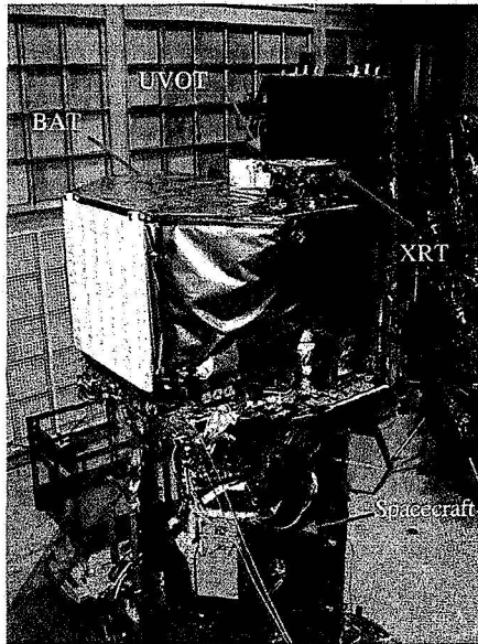
FIGURE 1.1. Left: The Swift Observatory in a class 10 000 cleanroom during the integration and test phase at the NASA/Goddard Space Flight Center. The three instruments are mounted on the optical bench with several of the electronics boxes and the sun-shield. The solar arrays are not yet installed. Right: Two typical GRB lightcurves in the pre-swift era, where there were limited observations of the GRB afterglow until around 10 000 seconds after the initial prompt gamma-ray emission.
