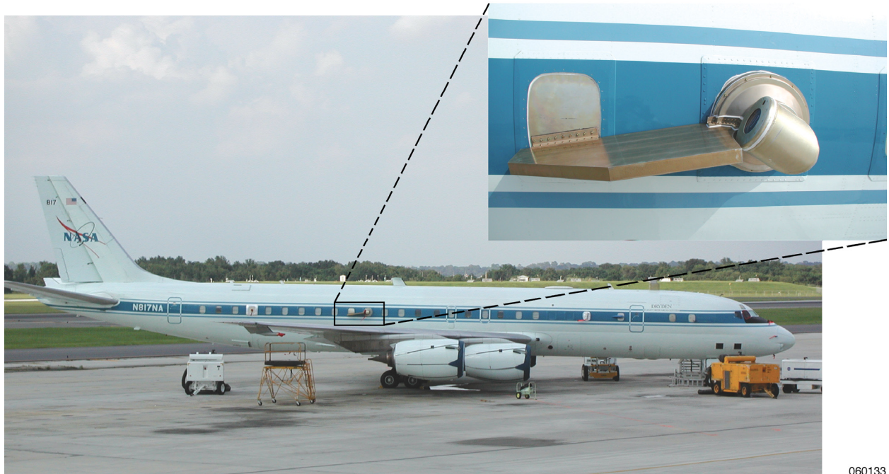
Figure 1. The lidar window assembly on the NASA Airborne Science DC-8 airplane; the rotating periscope is pointing toward the back, in the stowed position (inset).
