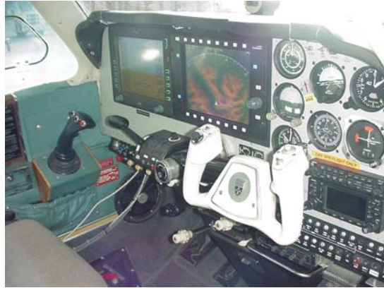
Figure 1 – Flight Deck of CJ-144. (Left side of cockpit is the EPS while the conventional instrumentation on the right side is used by the safety pilot.)
