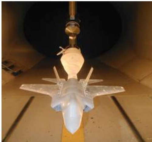
Figure 8. Test Model installed in the TDT
