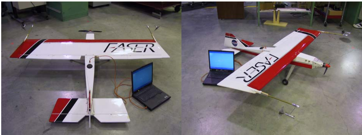
Figure 1 The FASER aircraft: Ultra Stick 120 with Ethernet connection of the laptop to the airplane shown.
