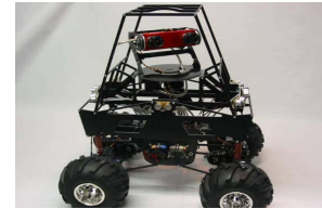
Figure 8. The MAX Rover hardware platform
