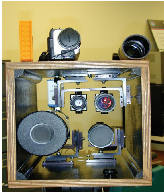
Figure 3. Tracker camera array fitted with lenses of various focal lengths and filters to reduce the daylight sky background.
