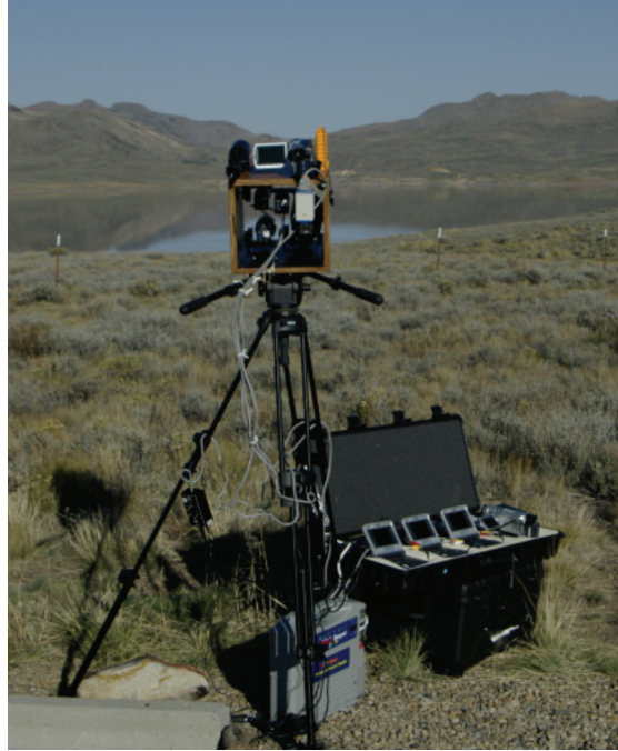
Figure 2. Tracker video array at Wild Horse, NV. Tracking was never achieved due to low visibility of the Genesis capsule.
