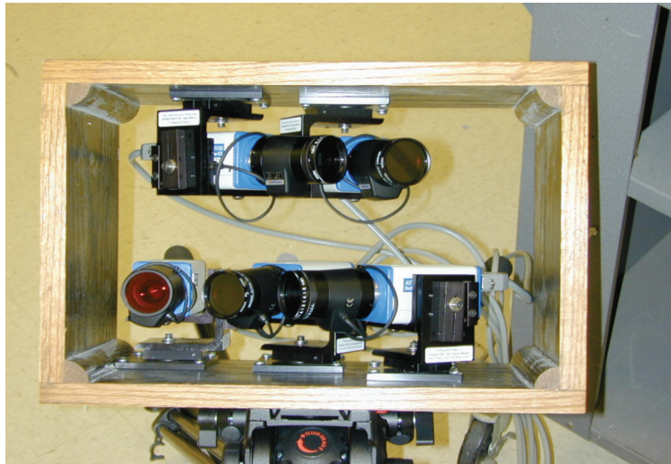
Figure 1. Mosaic camera array of five video cameras aligned to capture 110° FOV.
