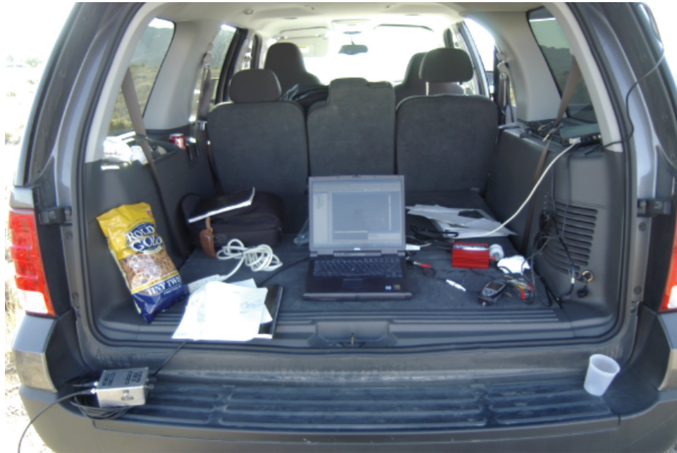
Figure 13. Laptop computer and PCR–1000 receiver (on shelf on the right) used to collect forward scatter radar data. A VLF receiver is visible at lower left.
