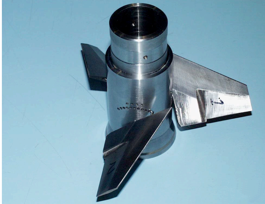
Figure 4. The modified tail-can of the three-percent-scale Hyper-X launch vehicle stack model with fin settings of 51 degrees.
