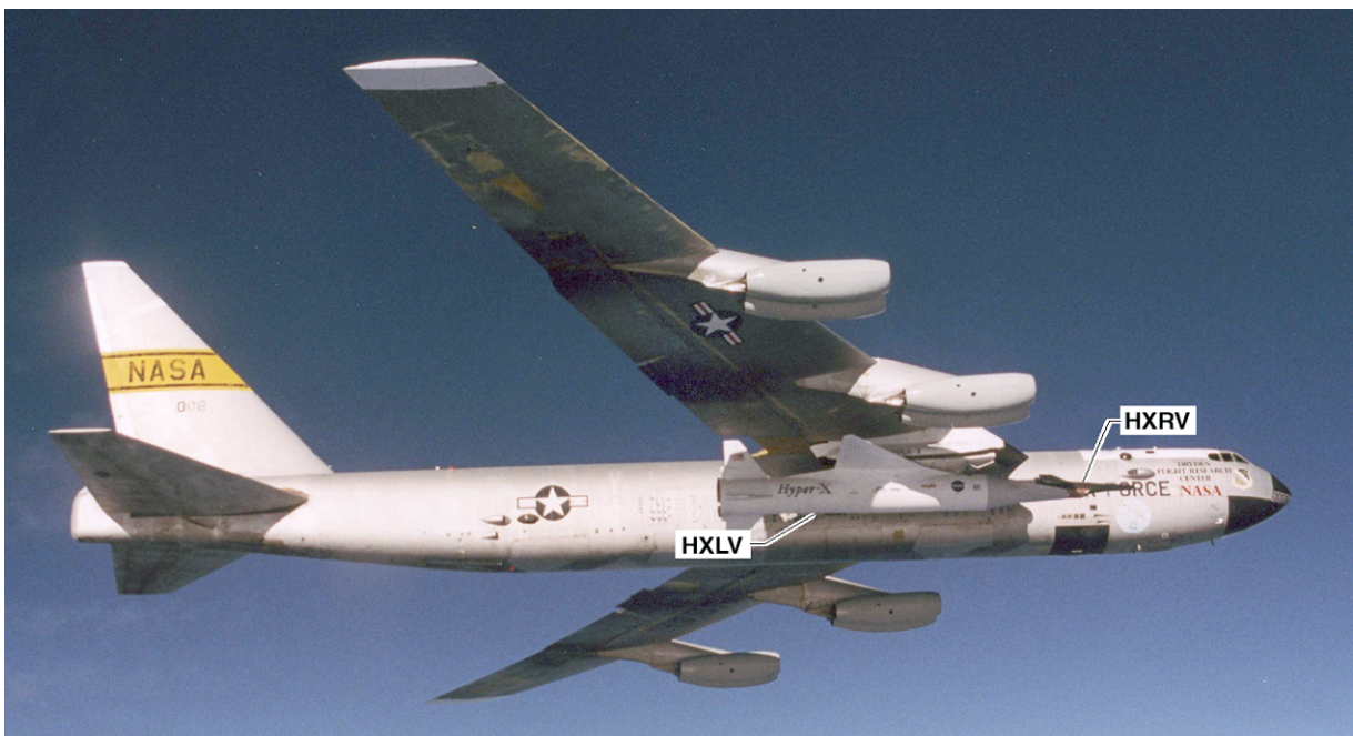
Figure 1. The B-52B airplane carrying the Hyper-X launch vehicle stack.
