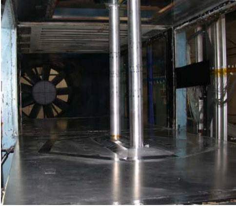
Figure 1. Tandem cylinder configuration in the BART facility.
