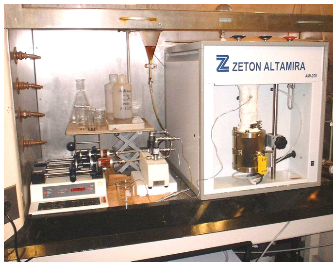
Figure 4.—Zeton-Altamira catalyst screening test rig.
