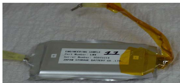
Figure 11. Laminate Pouch Cell after Overdischarge-into-Reversal Test.
