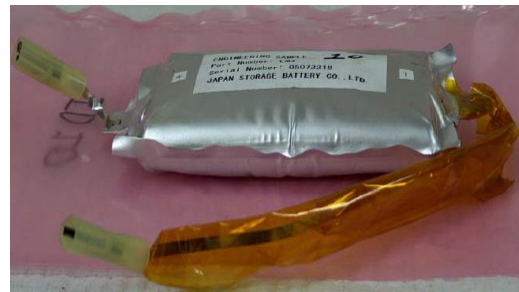
Figure 9. Laminate Pouch Cell Showing Expansion After Completion of Overcharge Test.
