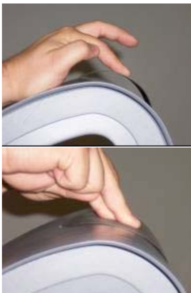
Figure 13. Plug flexes to conform to WLE panel.
