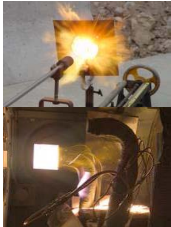
Figure 14. Typical torch and arc-jet tests.
