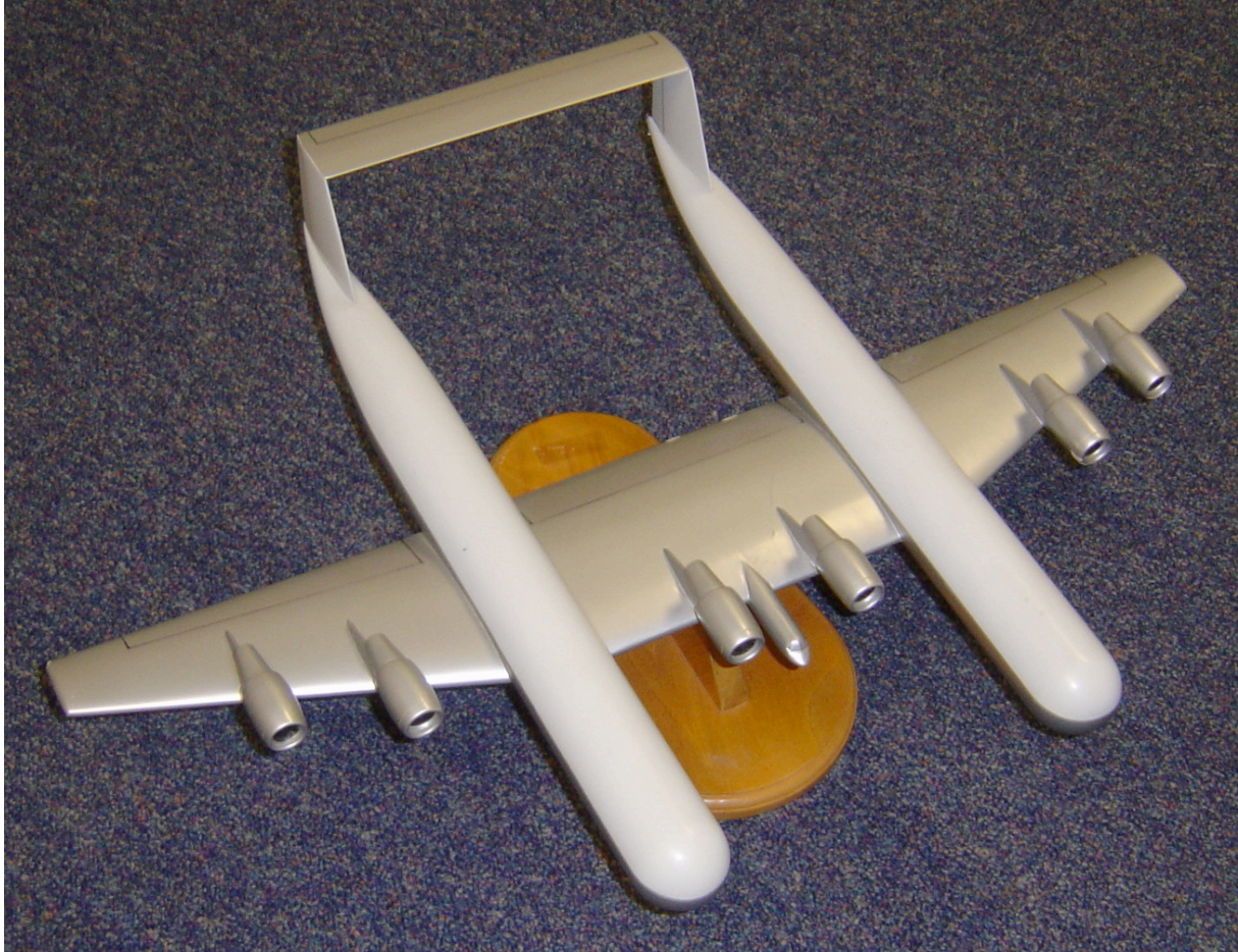
Figure 4. Model of very large catamaran aircraft studied by NASA. Note the cockpit between the two center engines.
