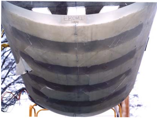
Figure 7. Post-test photograph of the bottom of the fuselage showing damage. The four dark regions are areas between the foam blocks.
