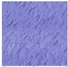
Figure 14(a): 2-D AFM scan of cantilever-beam based sensor after soaking in isopropyl alcohol.
