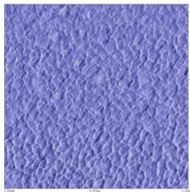
Figure 12(a): 2-D AFM scan of typical polymer-coated surface section of humidity Sensor. This scan has a dimension of 1.66 um x 36.7 nm.
