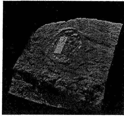
Figure 3. A 3-D model of the rock "King 3" at the MER-B landing site. The false color model was created from Pancam imagery, with a 3-D MI model superimposed over an area that was surfaced with the RAT.
