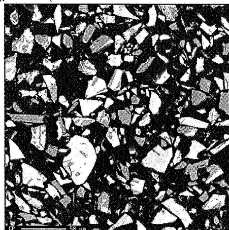
Fig. 2. BSE image of lunar simulant JSC-1AF fine fraction (polished mount). Grain size distribution of JSC-1AF has median size of \sim 25 \mu\text{m} from sieve analysis.
