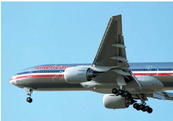
Figure 1. Deflected flaps/flaperons are typically in the jet exhaust plume or in the flow entrained by the jet during approach condition creating jet-flap interaction noise.
