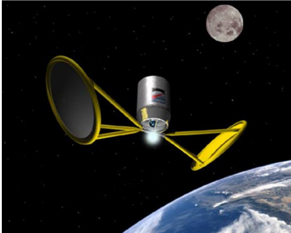
Figure 8. Application of the solar-thermal rocket for interorbit transfer.
