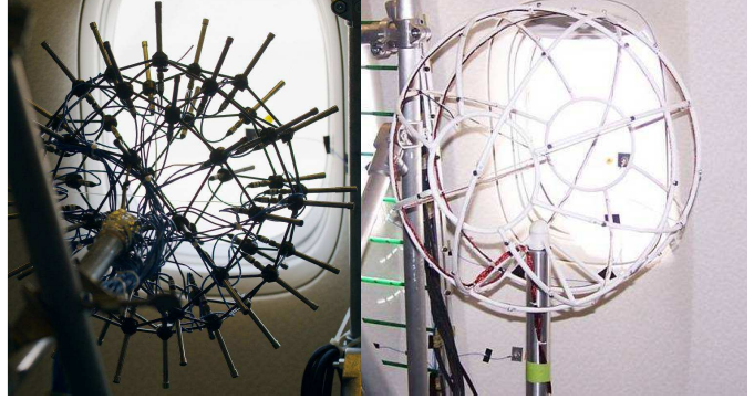
Figure 2. Two spherical array designs. The array on the left was design and build by the Naval Research Laboratory. The array on the right was designed and build by the Boeing ANP Laboratory.
