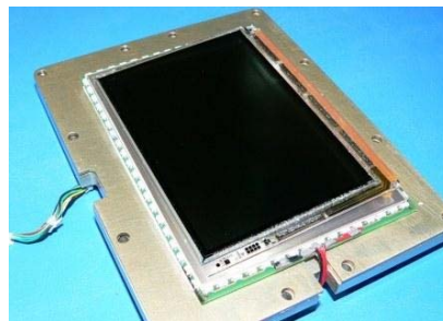
Figure 3. LED backlight replacing Fluorescent tube
