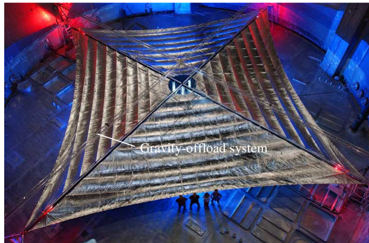
Figure 3. 20-m solar sail system tested at the NASA GRC Plum Brook Station Space Power Facility
