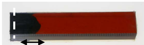
Figure 3. Plaque showing cut direction and MWCNTs alignment (arrow)
