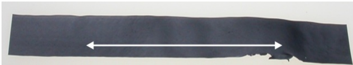
Figure 2. Ribbon of Ultem™/MWCNTs with arrow showing direction of tube alignment
