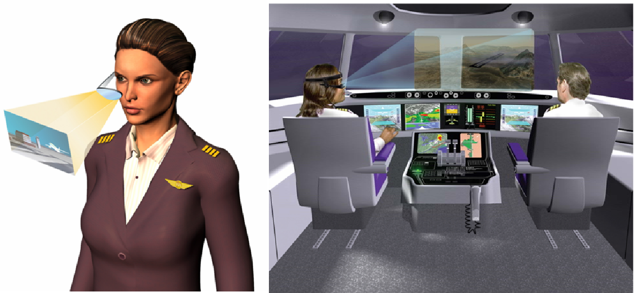
Figure 1: A Synthetic Vision enhanced HWD with a head tracker has unlimited field of regard.
