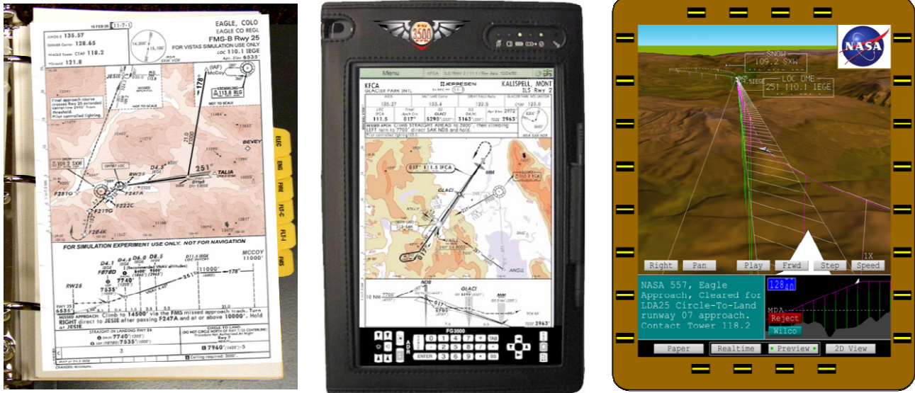
Figure 2: Paper charts (left), typical Electronic Flight Bag (middle) and the NASA-developed Mission Rehearsal Tool (right).
