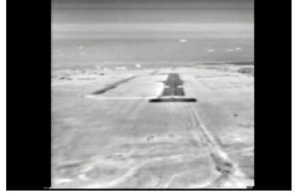
Figure 14. SWIR image from daytime flight. Note blooming in foreground. Figure 15. LWIR image from daytime flight. Figure 16. Enhanced, registered and fused output.
