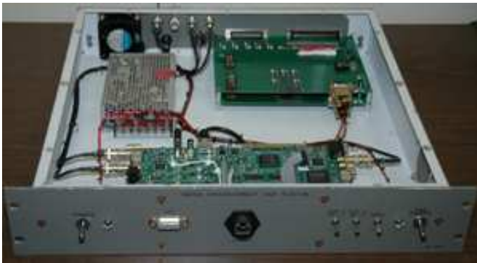
Figure 2. DM642 EVM, signal splitter boards, and power supply in flight box.
