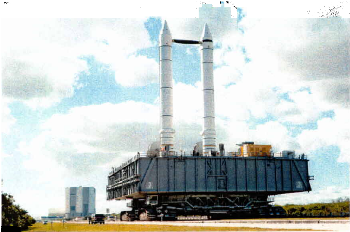
Figure 2. Partial Stack During Rollout Testing
