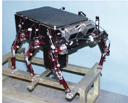
(b) First LEMUR Prototype Climbing.
