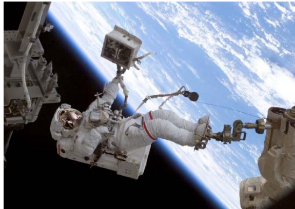
FIGURE 1. Astronaut David Wolf Riding the SSRMS End-Effector in a Foot Restraint on STS 112.
