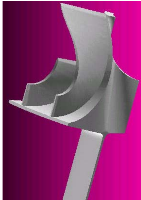
Figure 1.—Structural model for one blade passage (blade+splitter) of the BRU's radial inflow turbine.
