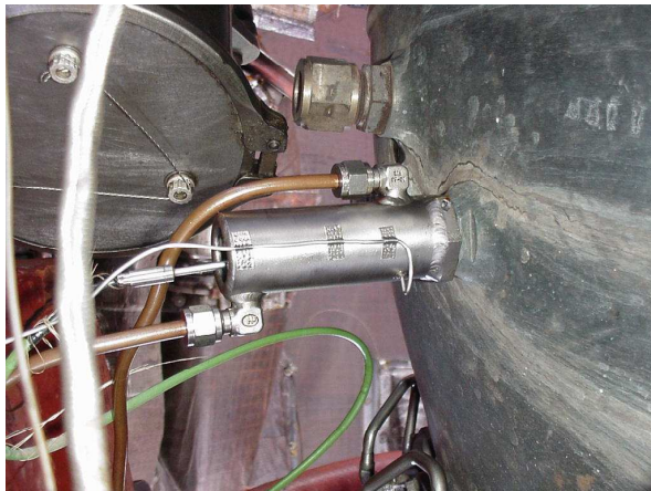
Figure 2. Kulite hardware mounted on PW4098 turbofan engine at Pratt & Whitney test stand C11, West Palm Beach Florida for EVNRC Phase 2 tests.
