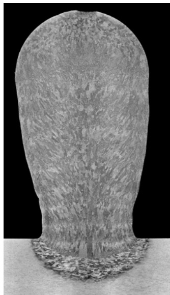
Figure 5. Microstructure for preheat pass plus 10 layers (20 kV accelerating voltage shown).
