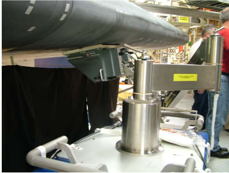
Figure 10 – Photograph of the manipulator system and the “right angle” hood/camera assembly performing an inspection in the OPF at KSC on the Space Shuttle Discovery following STS-114.
