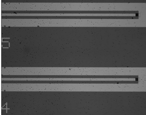
Figure 7.—Two photodetectors with their respective CPWs fully fabricated on the wafer.
