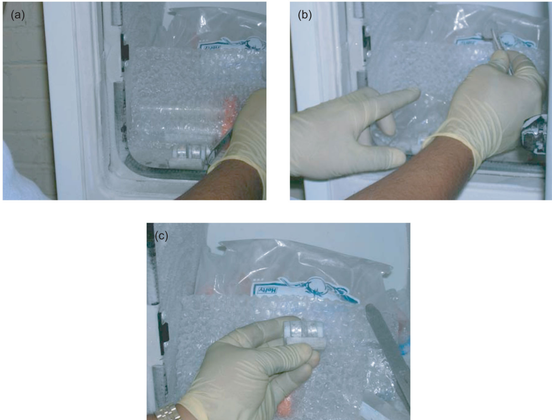
Figure 5.—Procedure for ice specimen pre-assembly with SHPB inserts. (a) Two aluminum inserts are positioned on Teflon (DuPont, Wilmington, DE) half-cylinder. (b) Ice specimen is taken out with tweezers and placed between inserts. (c) Final assembly.
