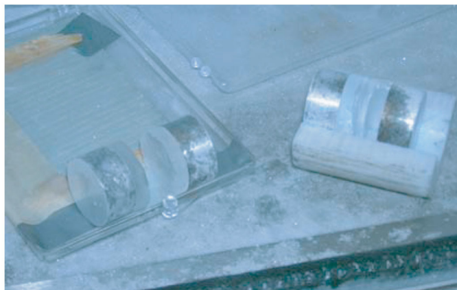
Figure 8.—Long ice specimens failed at midplane upon handling.
