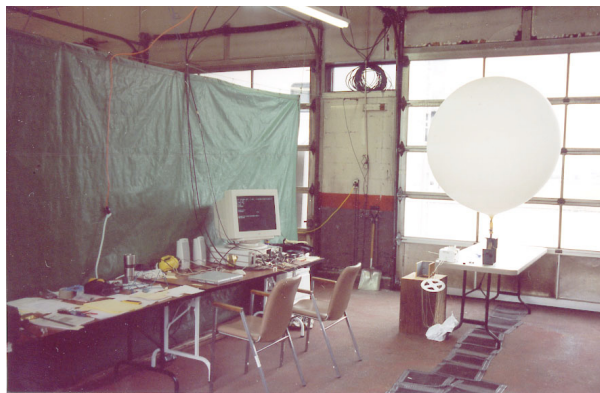
Figure 1, Balloonsonde system ready for launch, ground station and data acquisition system is on table at left.
