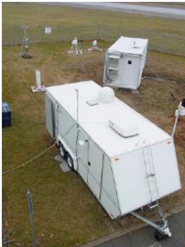
Figure 3, Remote sensing system deployed at Mirabel Airport. The radar dome is seen on the roof of the trailer in the foreground, with the ceilometer on the ground directly behind it. The two radiometers are at the center rear of the photograph.
