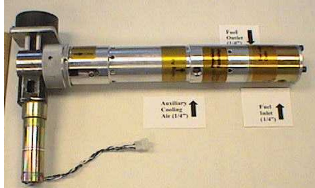
Figure 5.—A photo of the high-frequency “Georgia Tech valve” used for fuel-pulsing.
