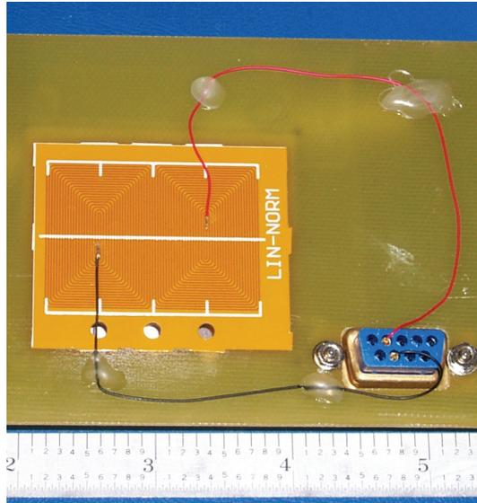
Figure 2. Sensor coil mounted to rigid base board.
