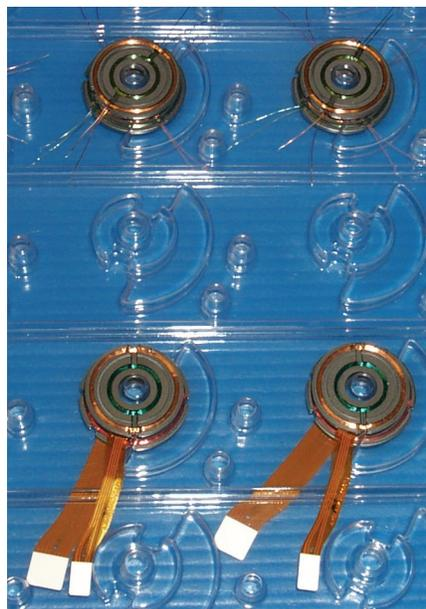
Figure 7. Multicoil rotary transformers.
