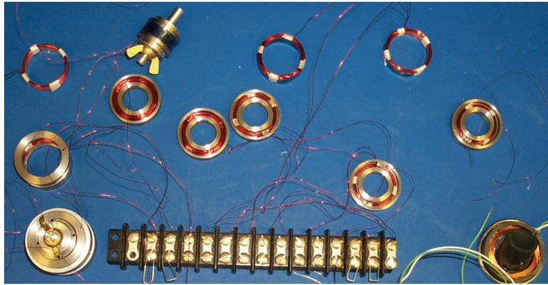
Figure 6. Rotary transformers.
