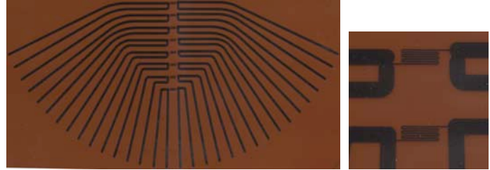
Figure 11. Laser-ablated thin-film resistance sensors on polyimide film.
