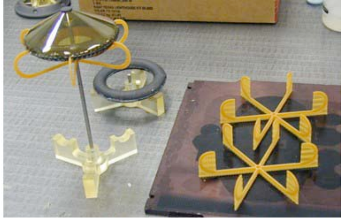
Figure 18. Temporary wax supports.
