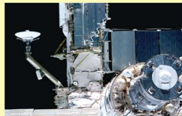
Backup 2-m inflatable Cassegrain reflector for ISS Ku-band system
