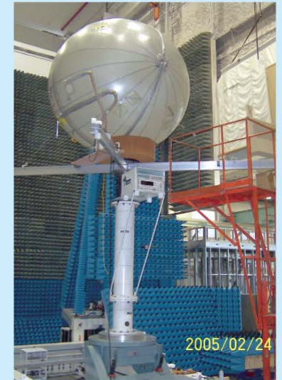
2.5-m inflatable membrane antenna in inflatable radome for ground applications
