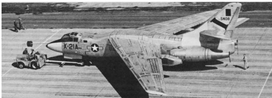
The Northrop-Air Force X-21A laminar-flow control research aircraft.
