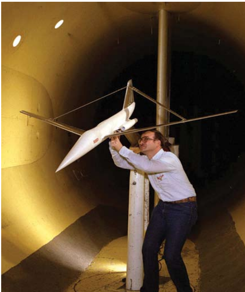
The 1/6-scale model of the Joined-Wing Research Aircraft in the Ames 12-Foot Pressure Tunnel.
