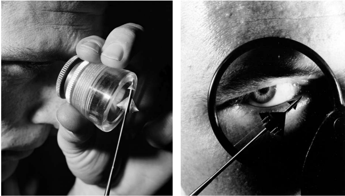
Small wind-tunnel models used in the Langley 4- by 4-Foot Supersonic Tunnel to study pressure fields associated with sonic booms.
