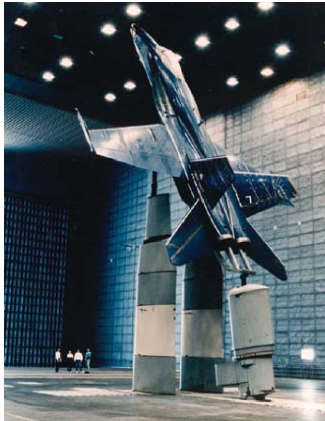
Supporting tests for the Actuated Nose Strake for Enhanced Rolling experiment included free-flight model studies (top) and tests on a full-scale F/A-18 in the Ames 80-by 120-Foot Tunnel (above).
