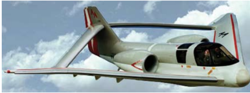
Boeing concept for a joined-wing flight demonstrator.
