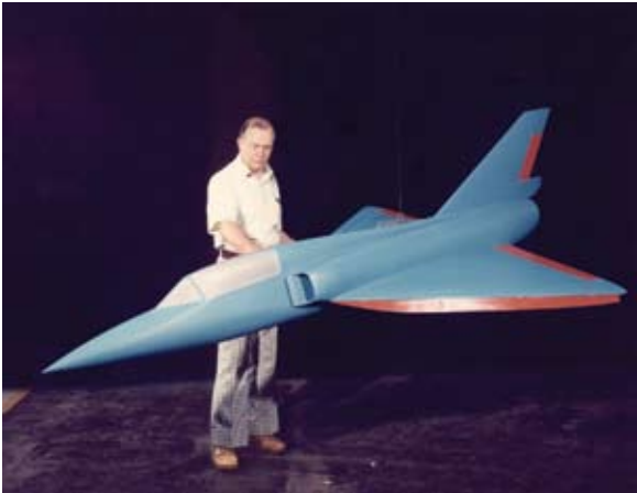
Free-flight model of the F-106B modified with a vortex flap (left) and in flight in the Langley Full-Scale Tunnel (right).
