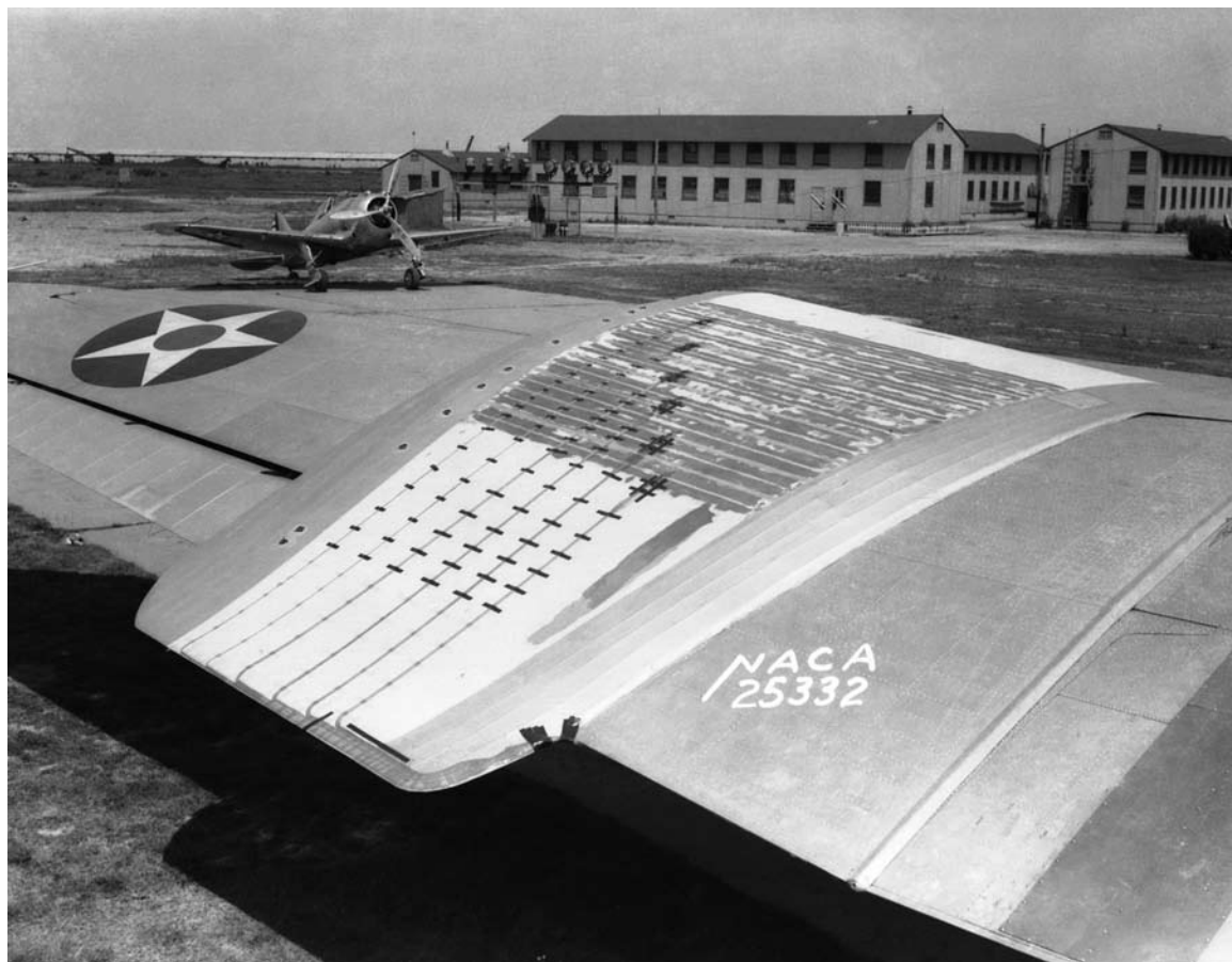
B-18 wing glove tests conducted by NACA (top) and close-up view of the glove panel used in natural transition studies (bottom).
