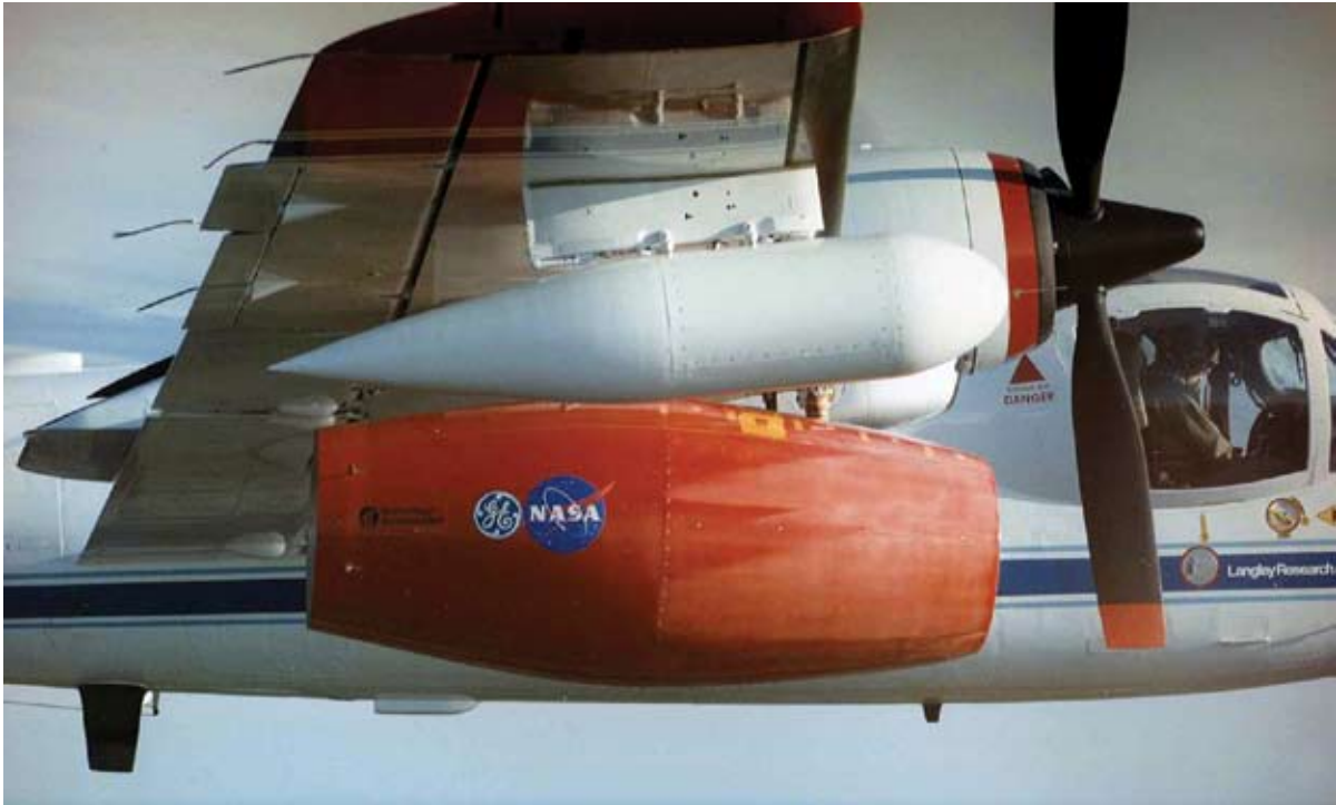
Sublimating chemicals indicate laminar flow (white area) on forward region of NLF nacelle during research flight.
