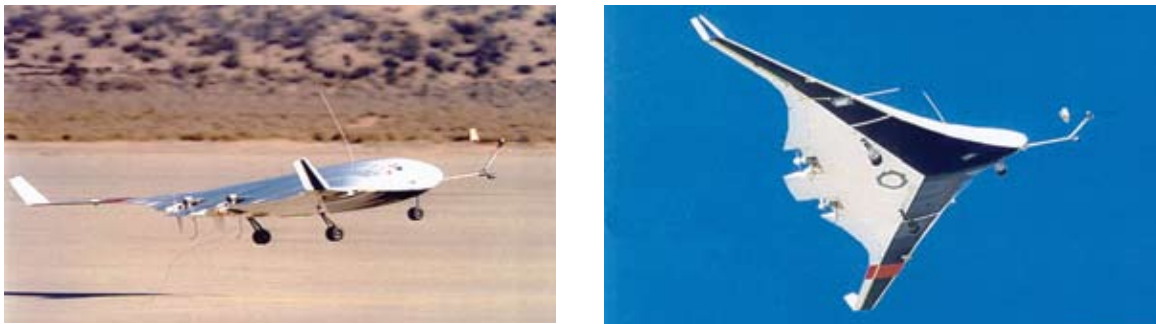
The 6-percent remotely controlled blended wing body model flown by the Stanford University Advanced Concepts for Aeronautics Program team.
