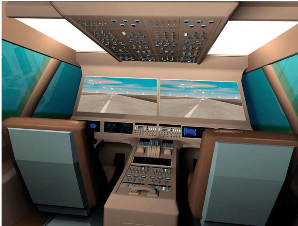
Conceptual synthetic vision system for a high-speed civil transport.
