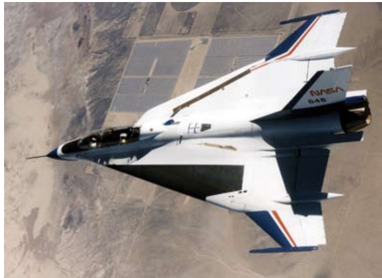
Modified F-16XL Ship 2 with supersonic laminar-flow glove installed in left wing panel.
