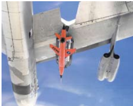
Drone with standard Firebee wing mated to B-52 in 1977 captive flight at NASA Dryden.
