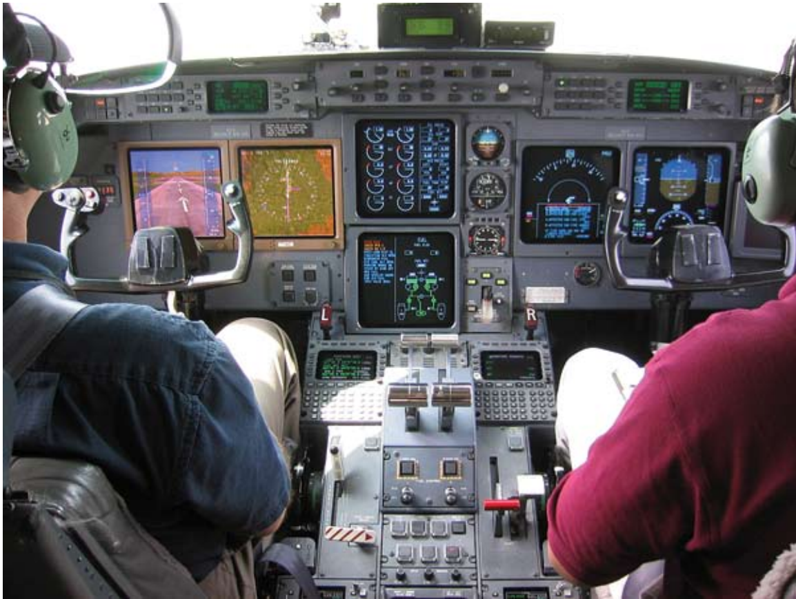
View of the synthetic vision system head-up and head-down displays (left) and the standard Gulfstream V display (right).
