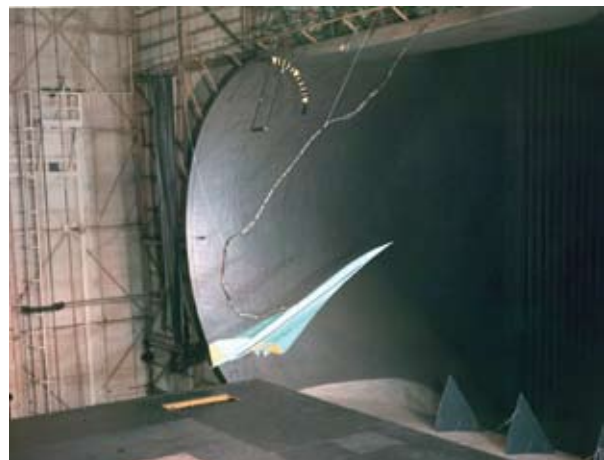
Researcher Delma C. Freeman, Jr., inspects a free-flight model of the Lockheed L-2000 Supersonic Transport design (left) used in tests in the Langley 30- by 60-Foot Full-Scale Tunnel.
