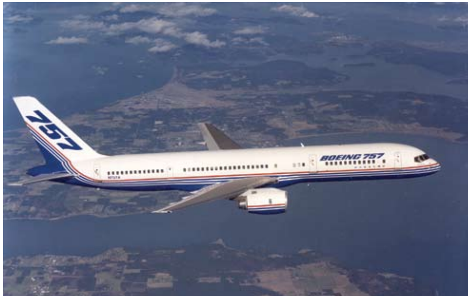
The prototype Boeing 757 transport used for the hybrid laminar flow control flight experiments.
