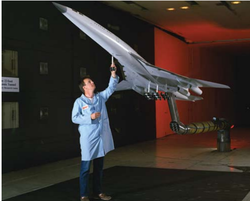
Technician Michael E. Ramsey inspects a 19-ft long model of the High-Speed Civil Transport Reference H configuration during tests of takeoff and landing characteristics in Langley's 14- by 22-Foot Subsonic Tunnel.
