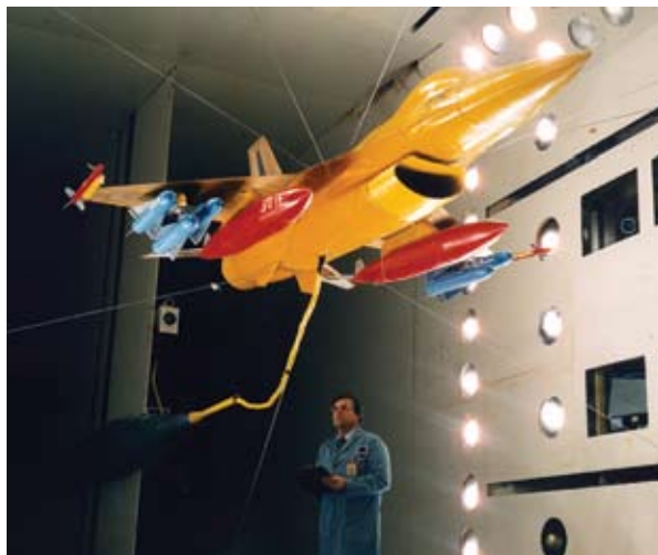
Jerome T. Foughner with F-16 model in Transonic Dynamics Tunnel during flutter tests with external stores.
