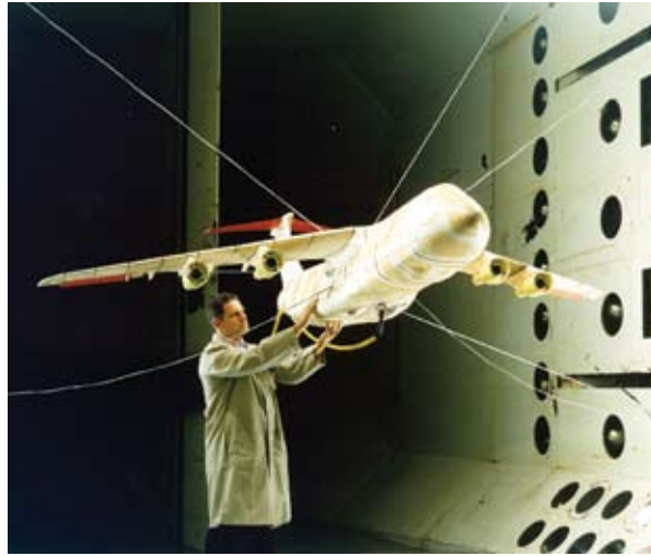
C-5 model mounted in the Transonic Dynamics Tunnel.
