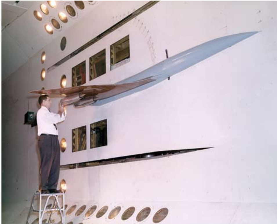
Charles L. Rublin inspects a 1/17-scale semispan flutter model of the Boeing 2707-300 during flutter clearance testing in the Langley 16-Foot Transonic Dynamics Tunnel in 1970.
