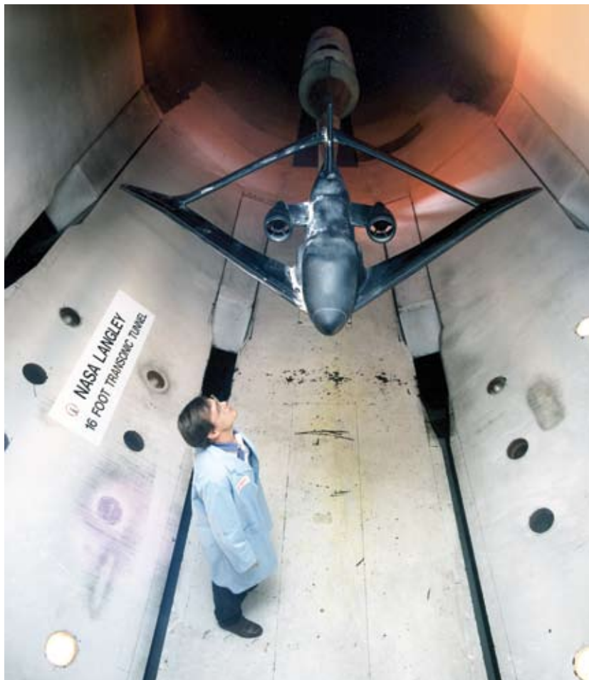
Jeff Yetter inspects the EX model in the Langley 16-Foot Transonic Tunnel in 1993.
