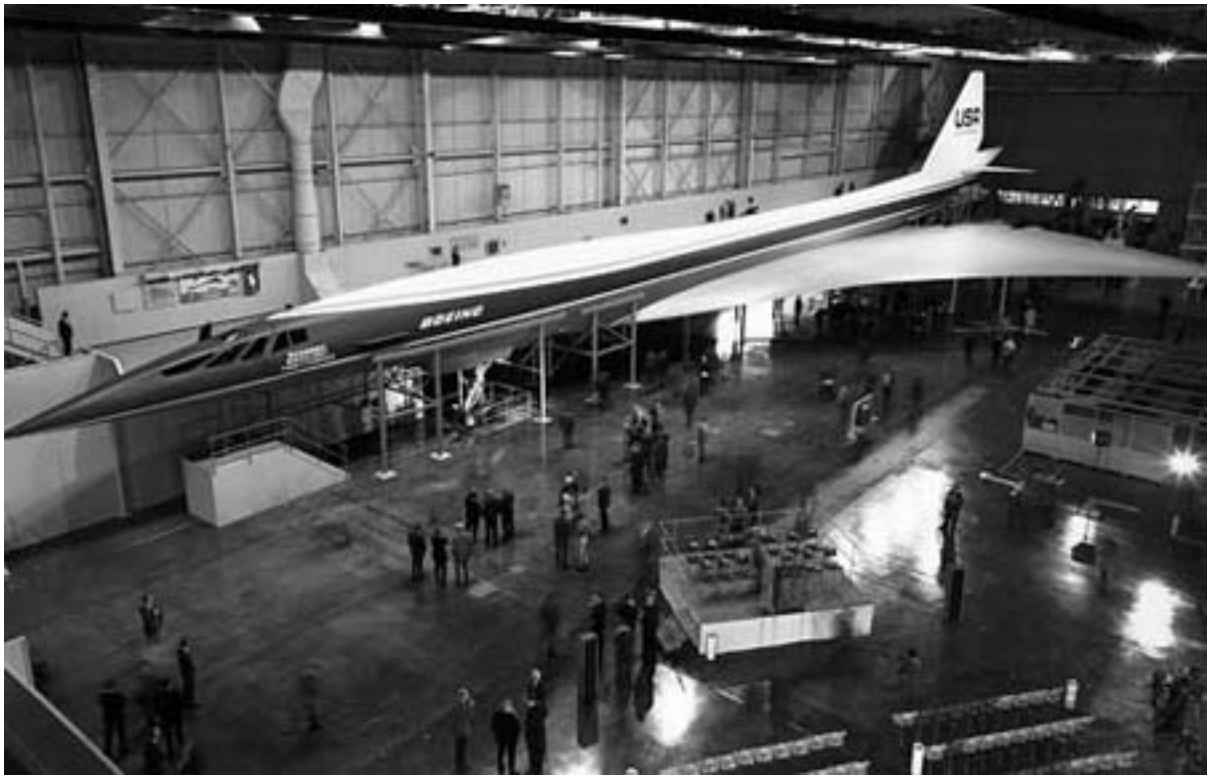
Engineering mock-up of the Boeing 2707-300 Supersonic Transport.
