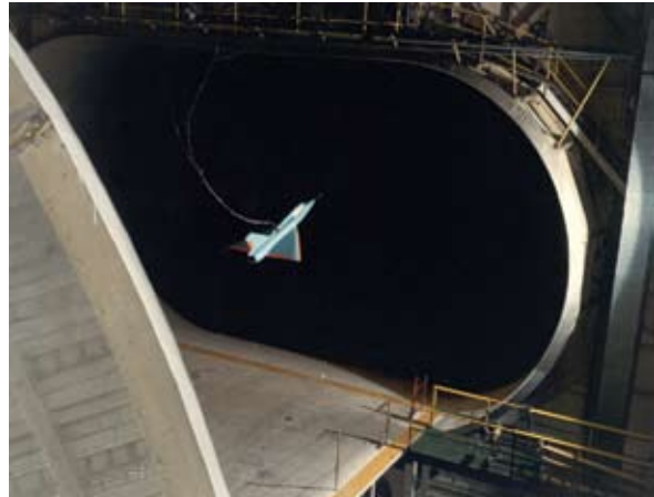
Free-flight model of the F-106B modified with a vortex flap (left) and in flight in the Langley Full-Scale Tunnel (right).
