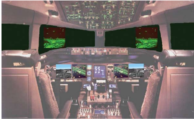
Conceptual head-up and head-down synthetic vision displays.
