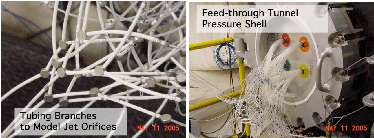
a) Splitting each actuator to multiple jet orifices
