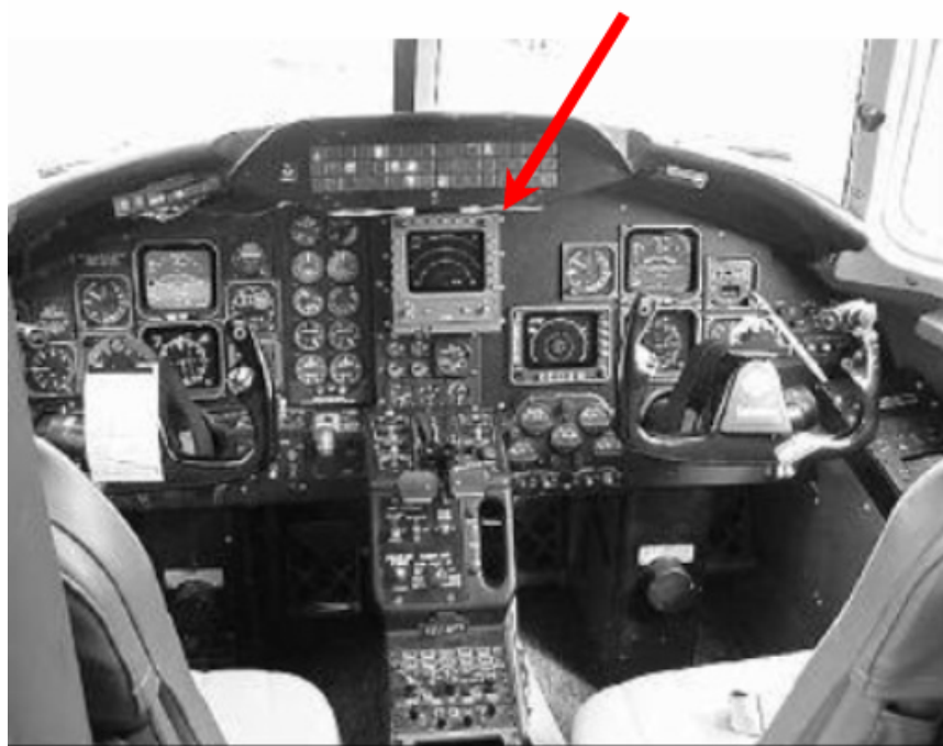
Figure 11. ATAAS Display Location on Rockwell-Collins Sabreliner
