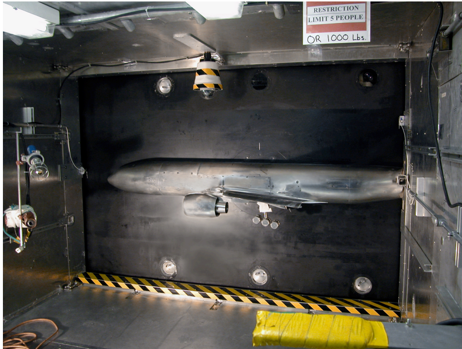
Figure 11. Photograph of modified access housing providing semi-span model access.
