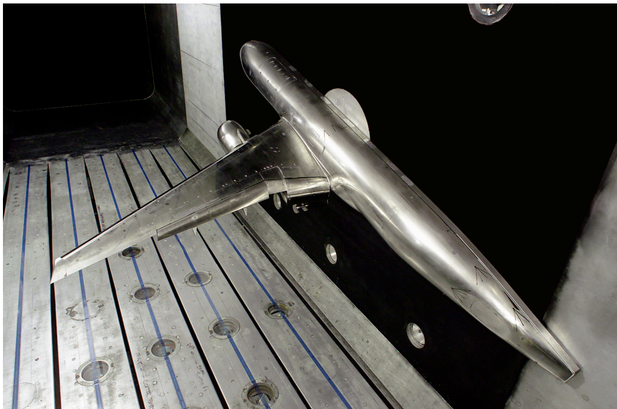
Figure 6. Photograph of a 5.2% Boeing 777 semi-span model mounted in the NTF.
